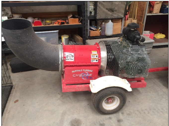
Leaf blowers can be extremely handy on prescribed fires – from backpack style blowers to the pull-behind style in the photo above (photo by M. Kline) – for quickly creating a bare soil firebreak in leaf litter.
